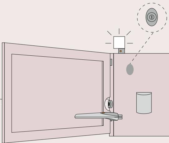
**1** Mount the brackets on the gate, observing the dimensions shown in the instructions
